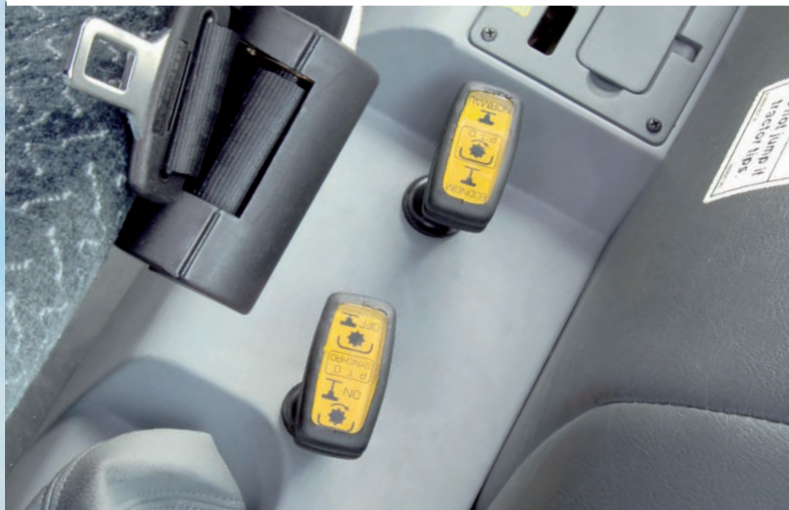
Four power take-off shaft speeds easily preselectable from the cabin.
