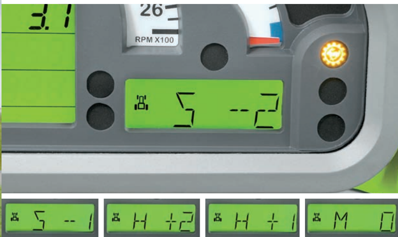
The indication for the group and gears is on the display.
