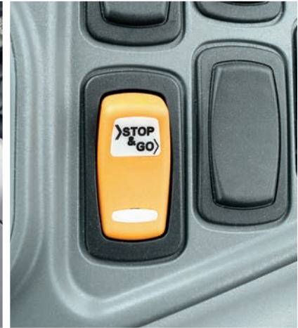
Stop & Go is activated per toggle switch.
