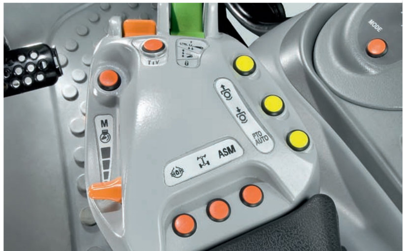
Electro-hydraulically operated PTO (push-button control).
