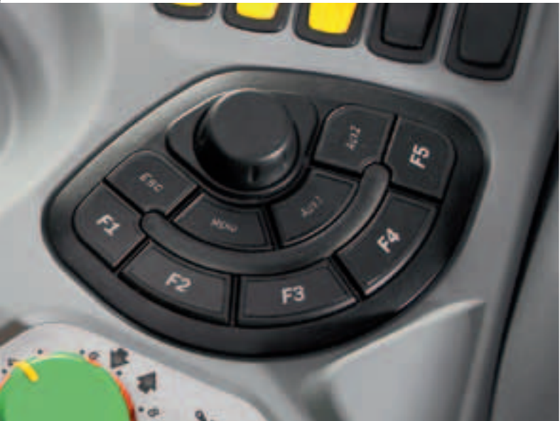
With the control panel located on a console to the right of the driving position, the operator can navigate easily through the menus using the dial.
