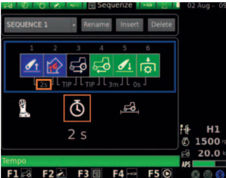
Thanks to the monitor, the management of the comfort tip allows up to 32 operations to be set and 100 different sequences to be stored.
