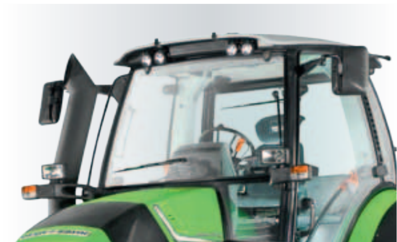
Twin pairs of lights incorporated at roof level, with extra wide beam provided by 14 powerful halogen lamps (Xenon lamps also available as optional accessory) able to illuminate a cultivation area of 600 m 2 .
