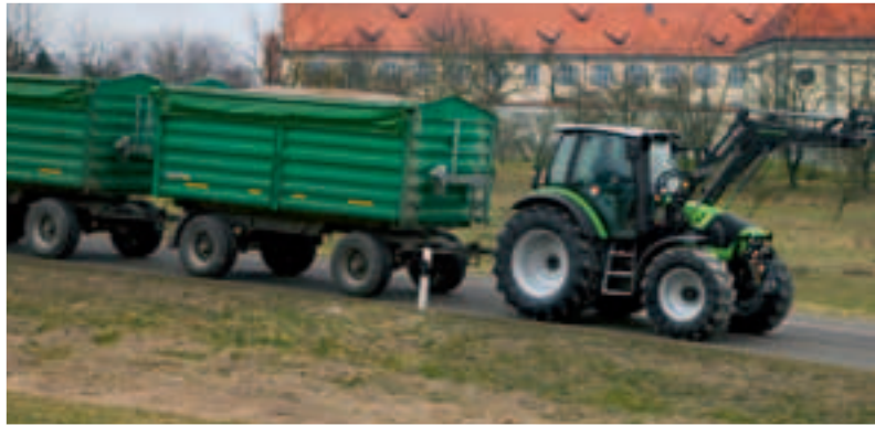
The TrailerStretch function, activated by a button in the cab, allows you to have a dual braking (transmission + brakes) in "Auto" mode.
