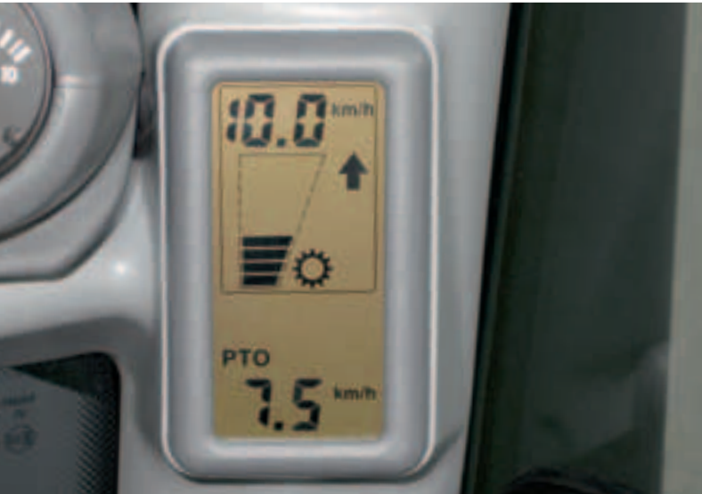
The PTO mode of the transmission is automatically activated when the PTO is engaged.
