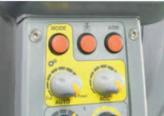
A button and two dials on the multifunction armrest are used to activate and control the various driving strategies, combining transmission and engine settings to best advantage.
