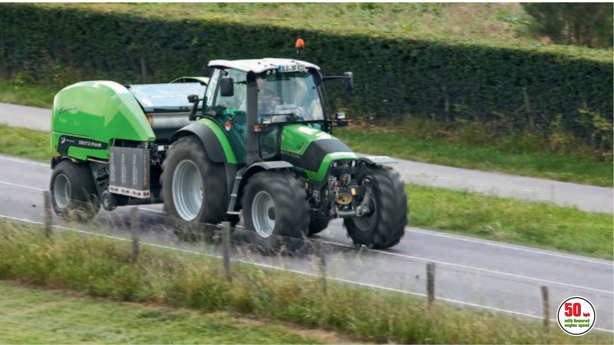
With the PowerZero function, the tractor can be held stationary on any terrain, regardless of gradient and load conditions.
