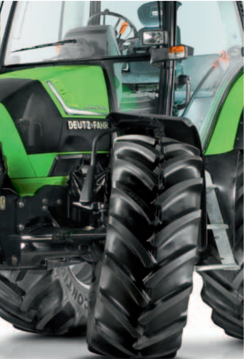
The trunnion mount creates a fulcrum coinciding with the centre line of the axle, allowing an oscillation of 22° at either end to negotiate even the roughest terrain.
