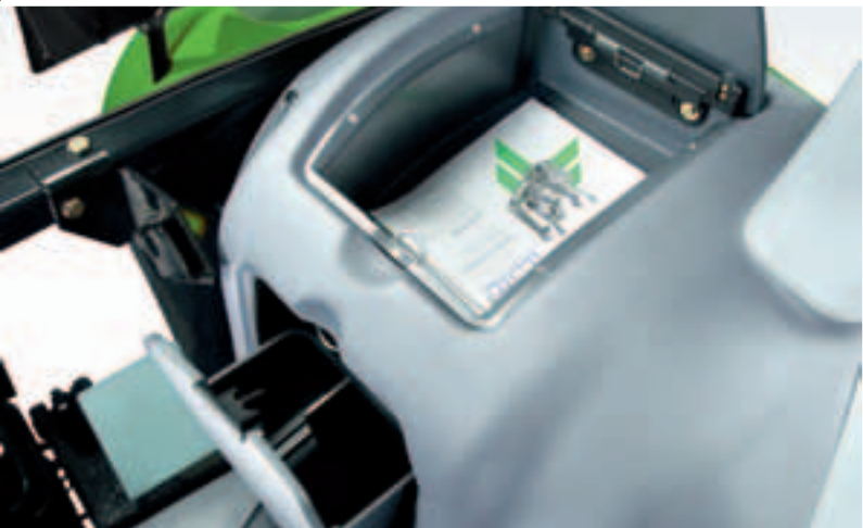
The drinks cooler compartment runs off the air-conditioning system and can hold 1 large bottle (2 litres) + 1 can. The storage compartment has a capacity of 7 dm 3 and will accommodate a DIN standard first aid box.
