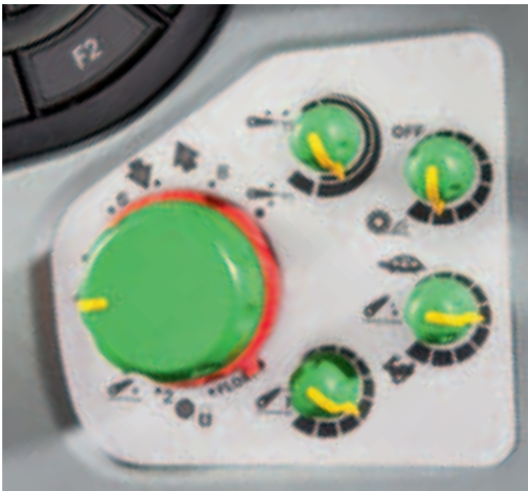
Lift movements and settings are selected from a side console and indicated by a digital display on the main instrument panel, in which the driver can view the various operating parameters.
