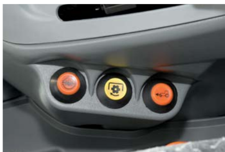
The differential locks can be activated at the touch of a button.
