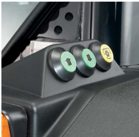
Everything to hand and in sight: the rear controls for the rear powerlift.
