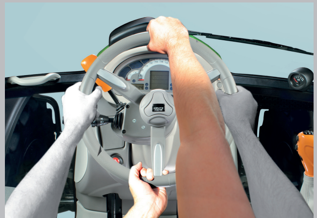
The SDD rapid steering system. Half the wheel rotation, double the steering power.
