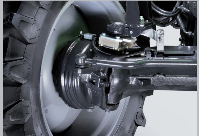
A unique safety concept from DEUTZ-FAHR. Separate oil cooled disc brakes on the front wheels.
