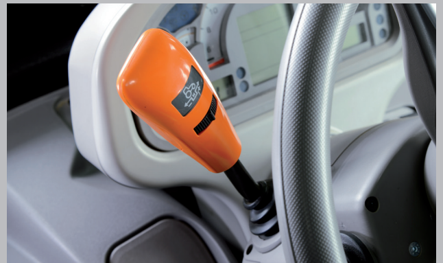
Powershuttle as standard. Electro-hydraulic reverse shuttle with adjustable five stage settings
