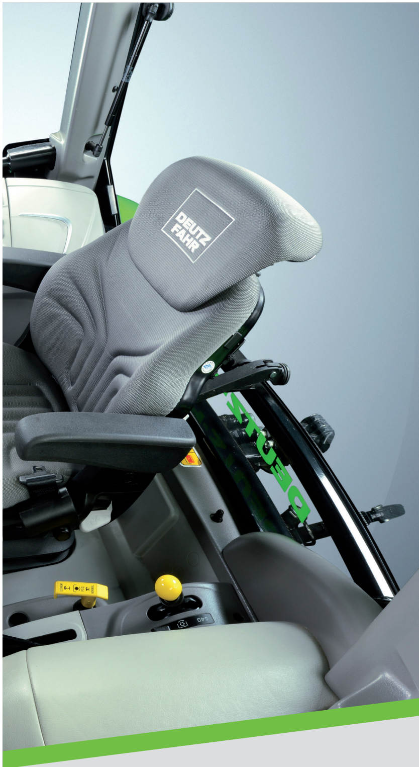
Cab vibrations reduced up to 40% thanks to "Hydro Silent-Block" suspension.
