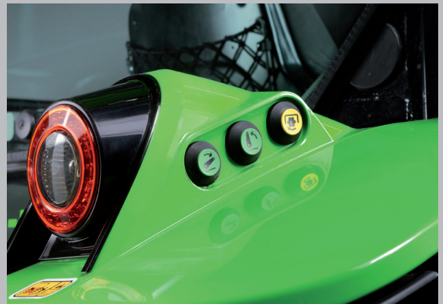
External PTO and rear lift controls for straightforward equipment mounting and external PTO operation.
