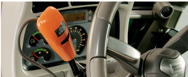
Powershuttle with SenseClutch function: 5 different levels of responsiveness, which can even be selected while on the move.
